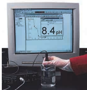
Figure 6.3 If the concentration of H_3O^+ or OH^- ions changes over the course of a reaction, a chemist can use a pH meter to monitor the reaction.
